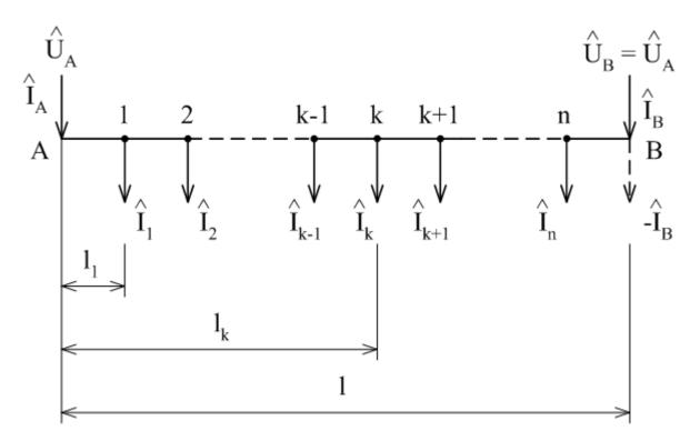
Calculation as for DC line (feeder is a negative load, zero voltage drop).
