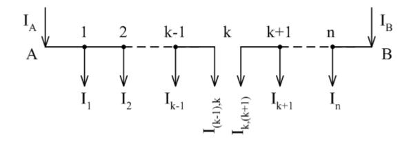
Single loads supplied from both sides – different feeders voltages
