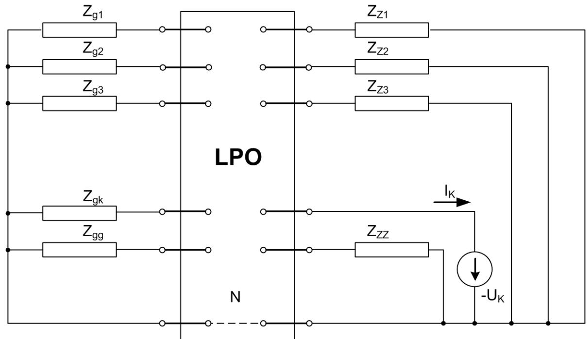
All node currents are zero except the short-circuit place, here an ideal voltage source → short-circuit admittance matrix.
