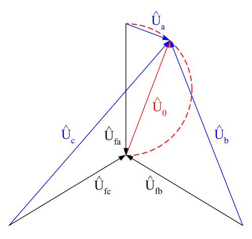
Disaffected phase voltage can be higher than the phase-to-phase value.
