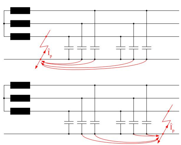
Note: overhead 22 kV – current c. 0,06 A/km cables 22 kV – current c. 4 A/km
