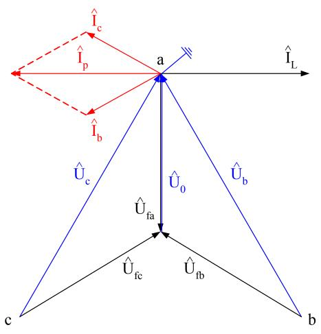
Fault current depends on the total system extent and almost doesn't depend on the fault point distance from the transformer.
