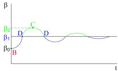
If the point C is too far ( $\Delta P$  accelerating)  $\rightarrow$  loss of synchronism.
