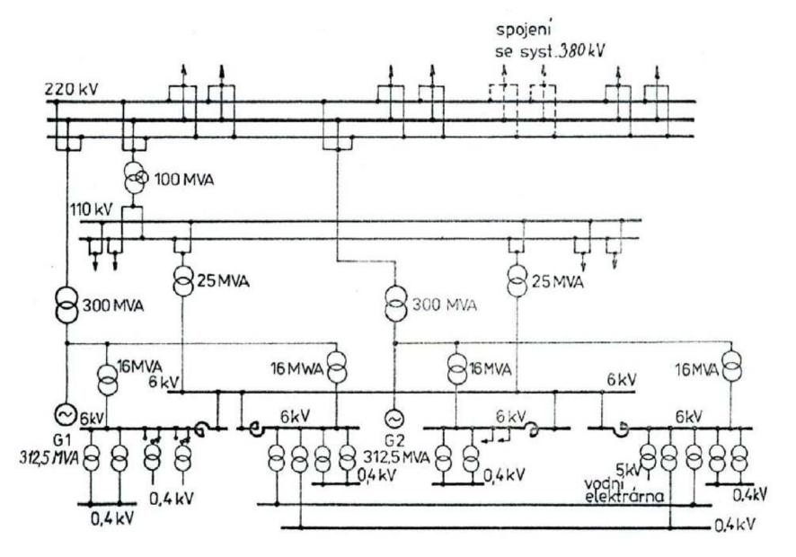
Typical CHP scheme with MV outlets to distribution network
