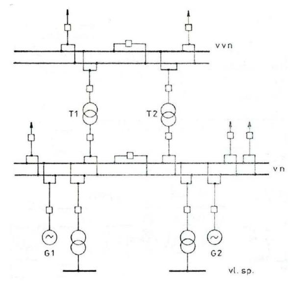
Alternative CHP scheme with MV outlets to distribution network with higher power output, short circuit currents are suppressed by reactors
