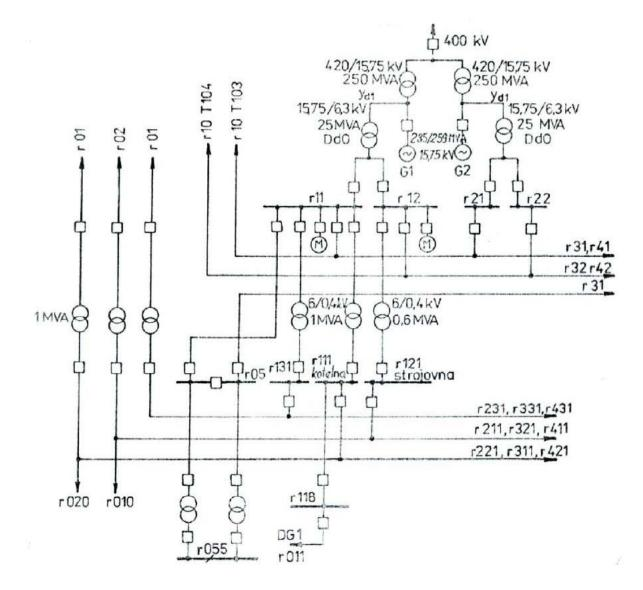
Conventional power plant, double unit 2x40 MW, Common aux. + diesel gensets
