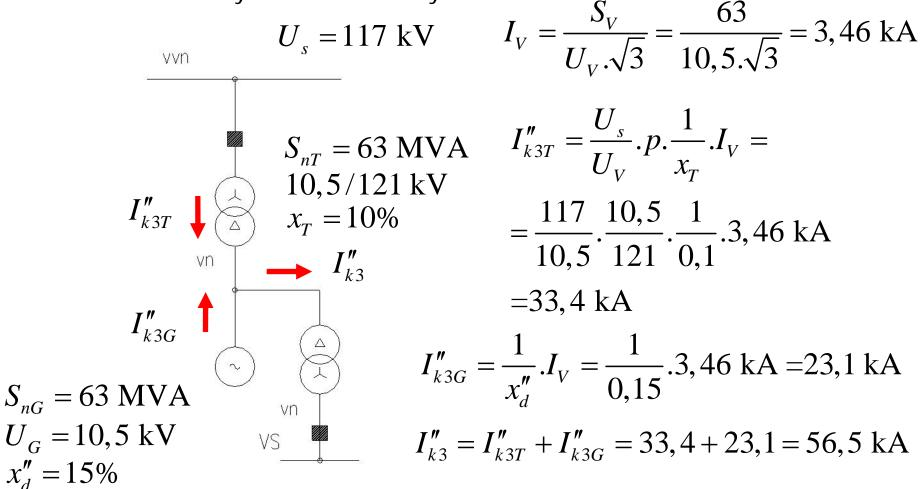
Initial short circuit current 56,5 kA in auxiliary is extremely high if we take into consideration normal operating current, in this case hundreds of amperes!
