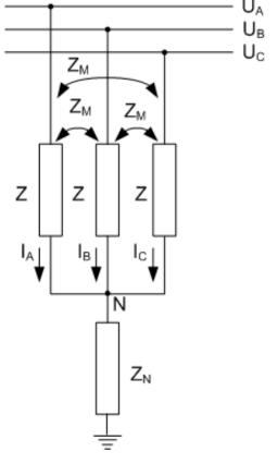
Symmetrical components voltages in the symmetrical segments depend only on the corresponding component current and component impedance.
