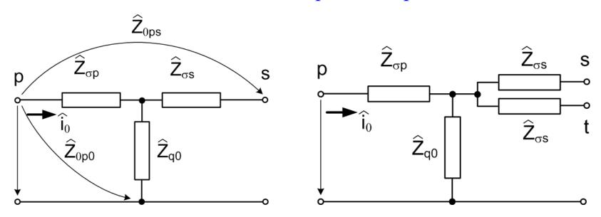
Series parameters are the same as for the positive sequence, the shunt always need to be determined.
