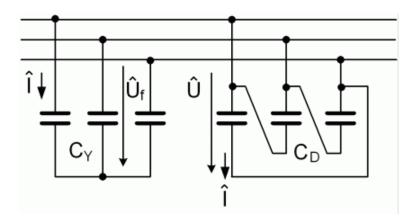
$$Q_f = U_f \cdot I_C = U_f^2 \omega C_Y \qquad Q_f = U \cdot I_C = U^2 \omega C_\Delta$$
