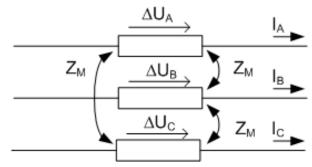
$$\begin{aligned} (\Delta U_{ABC}) &= (Z_{ABC})(I_{ABC}) \\ (T)(\Delta U_{120}) &= (Z_{ABC})(T)(I_{120}) \\ (\Delta U_{120}) &= (T)^{-1}(Z_{ABC})(T)(I_{120}) = (Z_{120})(I_{120}) \\ \hline (Z_{120}) &= (T)^{-1}(Z_{ABC})(T) \\ \hline (\hat{Z}_1 \quad 0 \quad 0) \quad (\hat{Z} - \hat{Z}' \quad 0 \quad 0) \end{aligned}$$
