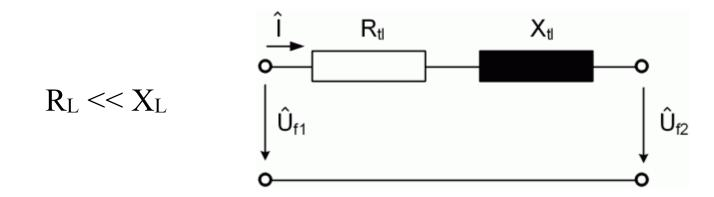
Input: X<sub>L</sub>%, S<sub>L</sub>, U<sub>n</sub>, I<sub>n</sub> Calculation:  $S_L = \sqrt{3}.U_n.I_n$   $X_L = \frac{X_{L\%} \cdot U_n}{100 \cdot \sqrt{3} \cdot I_n} = \frac{X_{L\%} \cdot U_n^2}{100 \cdot S_L}$   $\Delta \hat{U}_f = \hat{U}_{f1} - \hat{U}_{f2} = (R_L + jX_L)\hat{I} = \hat{Z}_L\hat{I}$   $\hat{Z}_{Labc} = \hat{Z}_L \cdot [E] - 3ph \text{ inductor}$  $\rightarrow \text{ self-impedance } \hat{Z}_L, \text{ mutual impedances } 0$
