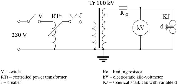
Tr - testing transformer 100 kV
