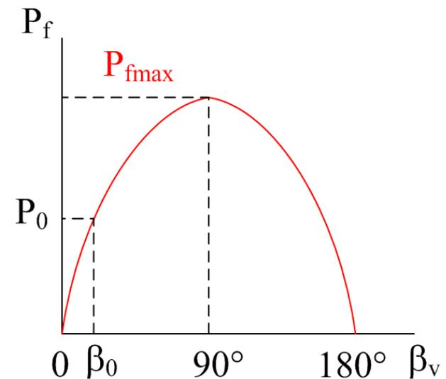
In addition to power lines also reactance of generators, transformers ... are added  $\rightarrow$  higher power angle. Generators have the biggest influence (X).
