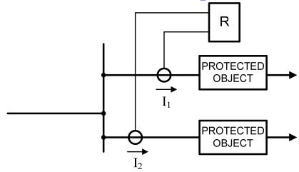
e.g. as the generator turn protection (stator winding of 2 parallel branches)
