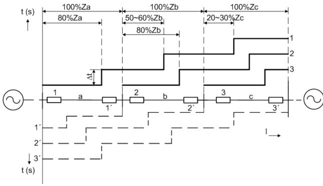
$$1^{st} \ level: \quad 0.8 \ z_a \\ 0.01 - 0.02 \ s \ (immediate) \\ 2^{nd} \ level \quad 0.8 (z_a + 0.8 \ z_b) \\ 0.6 \ s$$
