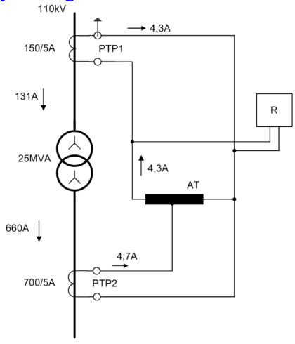
b) unequal CT construction – different overcurrent numbers
