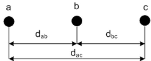
The power line is asymmetrical and non-transposed so operational inductances of each phase are different and moreover complex.
