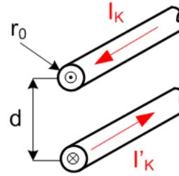
**3) total inductance of one conductor in a loop**
