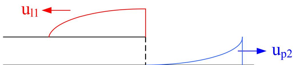
Note: Longitudinal inductance has the same characteristics as cross capacity. Cross inductance has the same characteristics as longitudinal capacity.
