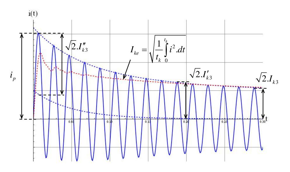
Calculation of peak short circuit current acc. to EN 60 909-0:
