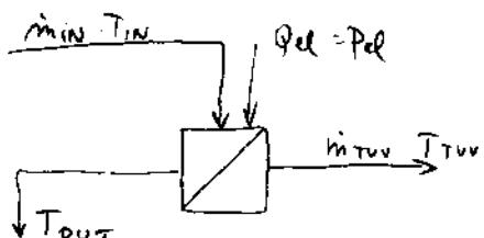
$$\dot{m}_{IN} \cdot C_p_{UV} \cdot (T_{IN} - T_{OUT}) + Q_{el} = \\ = \dot{m}_{TUV} \cdot C_p \cdot (T_{UV} - T_R)$$
