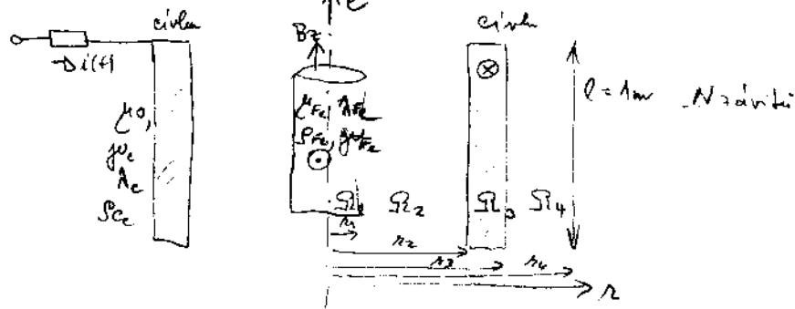
$$rot H = J \quad rot E = -\frac{\partial B}{\partial t} \quad B = \mu H \quad \nabla \times \frac{J}{\rho \mu_0} = -\frac{\partial B}{\partial t}$$
