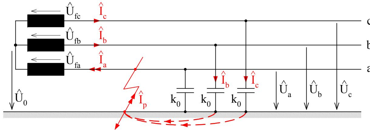
Fault current composed of 2 capacitive currents in the disaffected phases.
