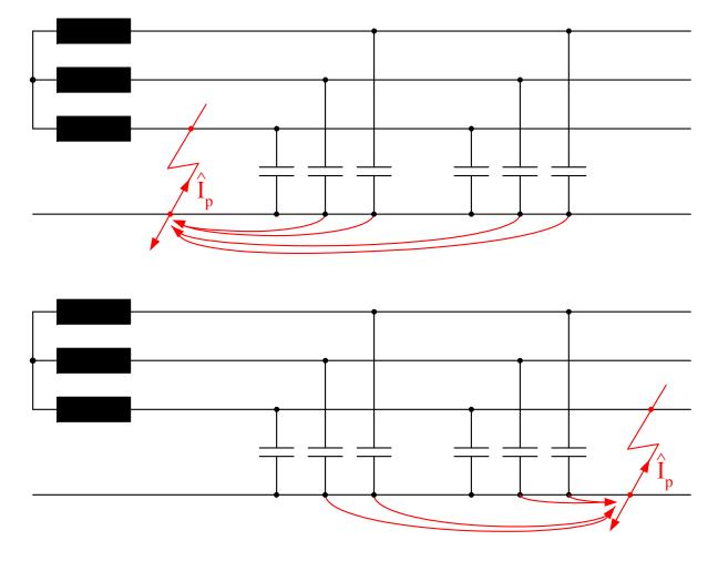
Note: overhead 22 kV – current c. 0,06 A/km cables 22 kV – current c. 4 A/km
