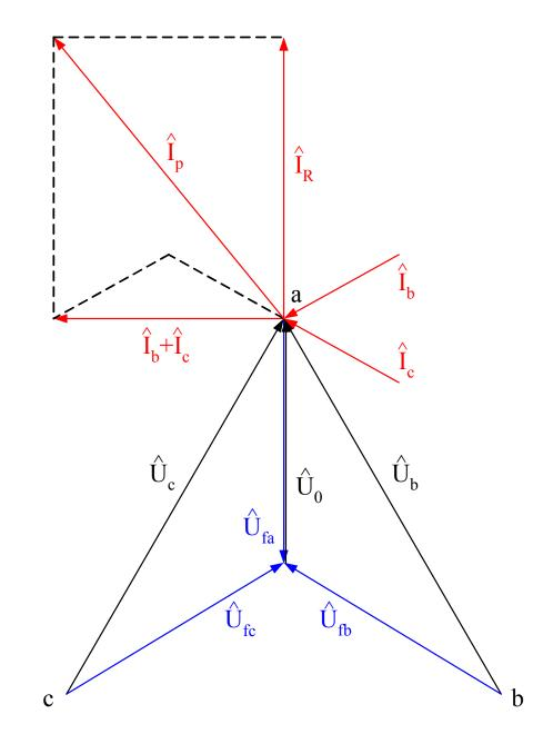
Neutral point voltage in a faultless state  $(k_{b0} = (1 - \Delta)k_{c0}; k_{a0} = k_{c0} = 50 \cdot 4 \text{ nF} / \text{km} \cdot 50 \text{ km})$  $R_{uz} = 20 \Omega$
