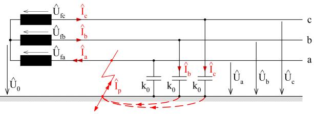
Fault current composed of 2 capacitive currents in the disaffected phases.
