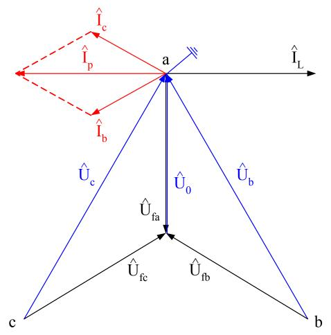
Fault current depends on the total system extent and almost doesn't depend on the fault point distance from the transformer.
