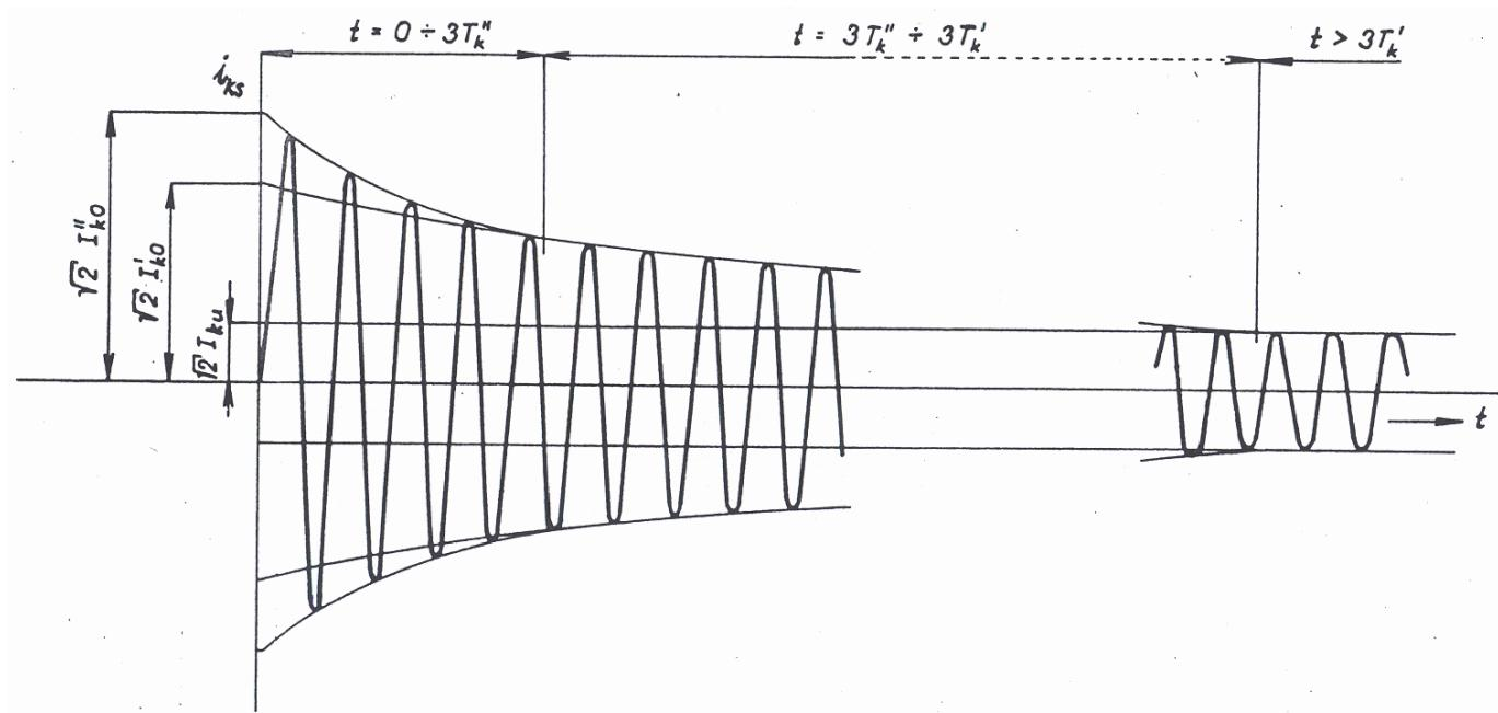
Short-circuit components ( $f = 50$  Hz):
