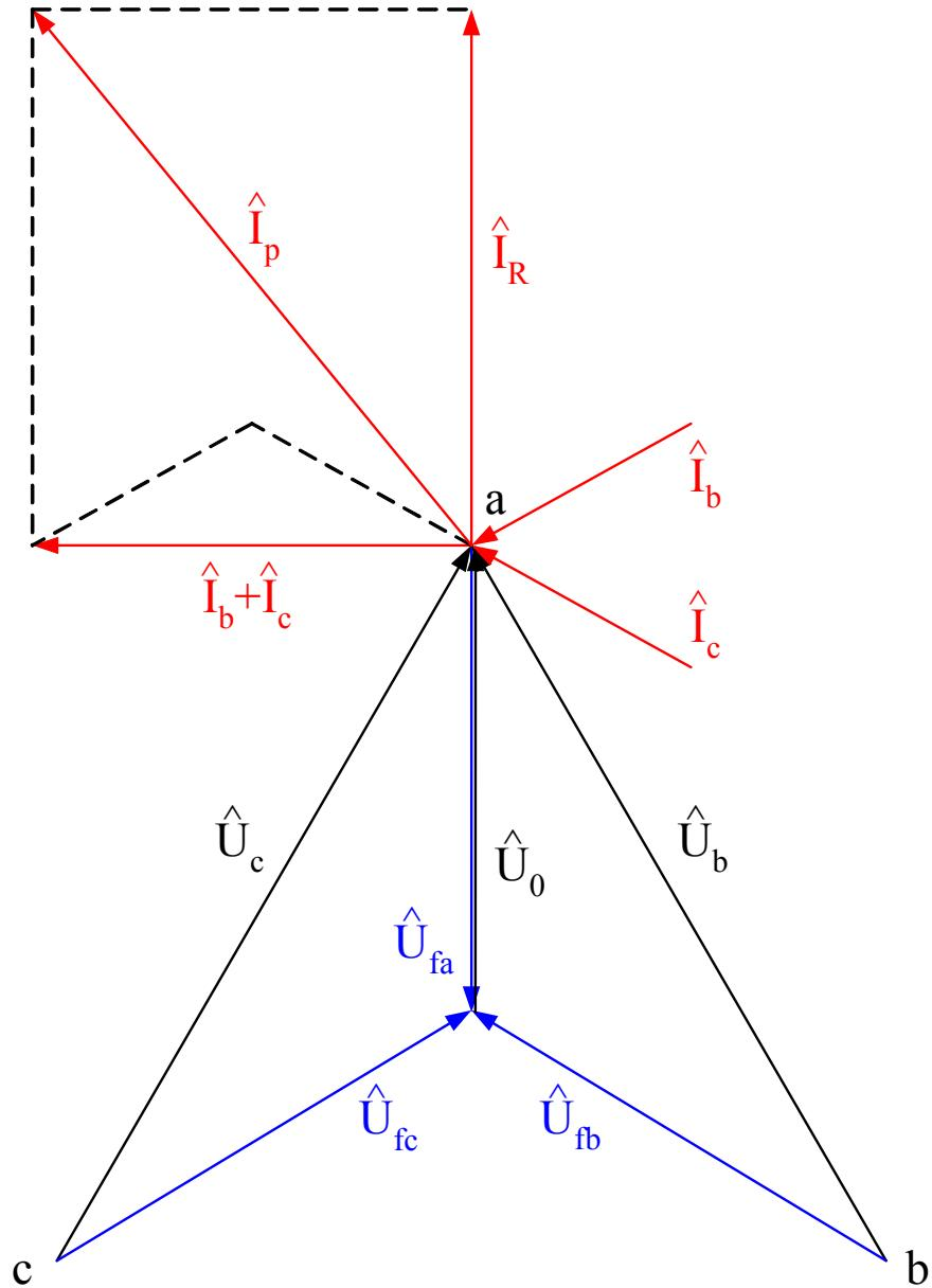
Neutral point voltage in a faultless state
