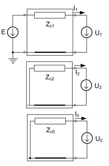
Three-phase (to-ground) short-circuit
