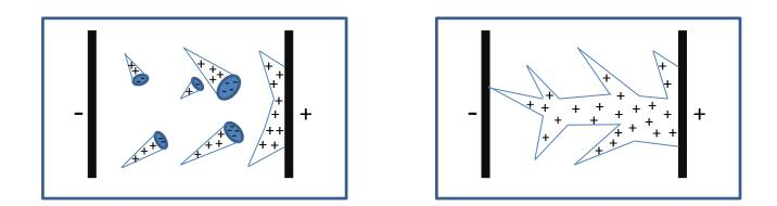
After the primary avalanche is passed through the area between electrodes the ionized channel remains and the main discharge then occurs.
