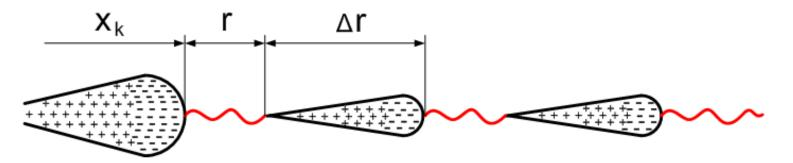
The velocity of electrons propagation is then  $\frac{r+\Delta r}{\Delta r}$ times higher than the velocity of electrons in avalanche
