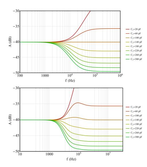
Attenuation of RC divider for various capacitors  $C_2$ , the divider is fully compensated when  $C_2$ =100 pF
