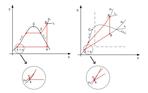
**Process k-n:** The working fluid (general water) is pumped from low to high pressure. As the water is liquid at this stage, the pump requires little input energy. Usually this process is neglected for calculation of thermodynamic efficiency.
