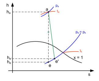
The non-ideal emission enthalpy  $h_e$  can be calculated from the turbine thermodynamic efficiency formula:
