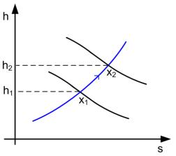
Dryness of wet steam - the ratio of steam content and the total mixture of steam and water:
