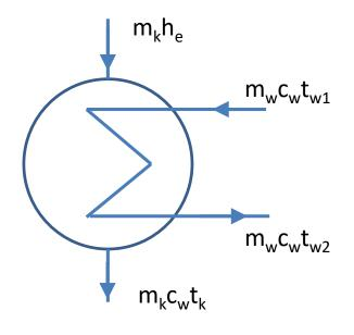
$$m_k h_e + m_w c_w t_{w1} - m_w c_w t_{w2} - m_k c_w t_k = 0$$
