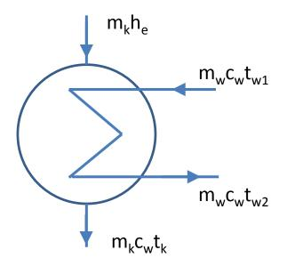
$$m_k h_e + m_w c_w t_{w1} - m_w c_w t_{w2} - m_k c_w t_k = 0$$
