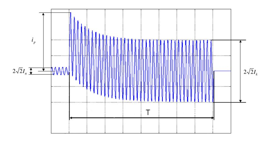
$I_p$  – peak short circuit current,  $I_k$  – steady state short circuit current
