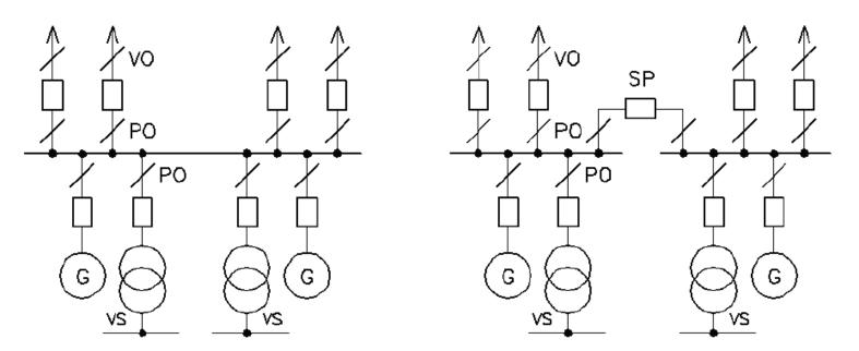
VO – feeder disconnecter, PO – Bus-bar disconnecter, VS – bus-bar of self consumption, G – generator unit, SP – Bus – bar circuit breaker **Electrical Parts of Power Plants**
